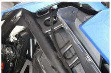
Open the Dash storage and remove the tray, run the harness up into the compartment.
