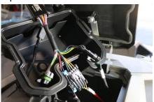
Go up the fender support into the dash. Plug into the Control Module.
