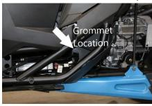
Run the rear harness from the taillight down along the frame to the main wire harness where there is a large rubber grommet behind the OEM battery relay going through the rear fire wall, push the connector through the grommet.
