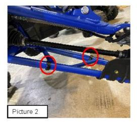
C. Once Place the Driver side a-arm guard (HTRFLV-DF) on the Driver side a-arm. Then when aligned place (2) M6 x 40mm bolts and (2) bowl washers in the locations shown in (Picture 3). Loosely tighten.
