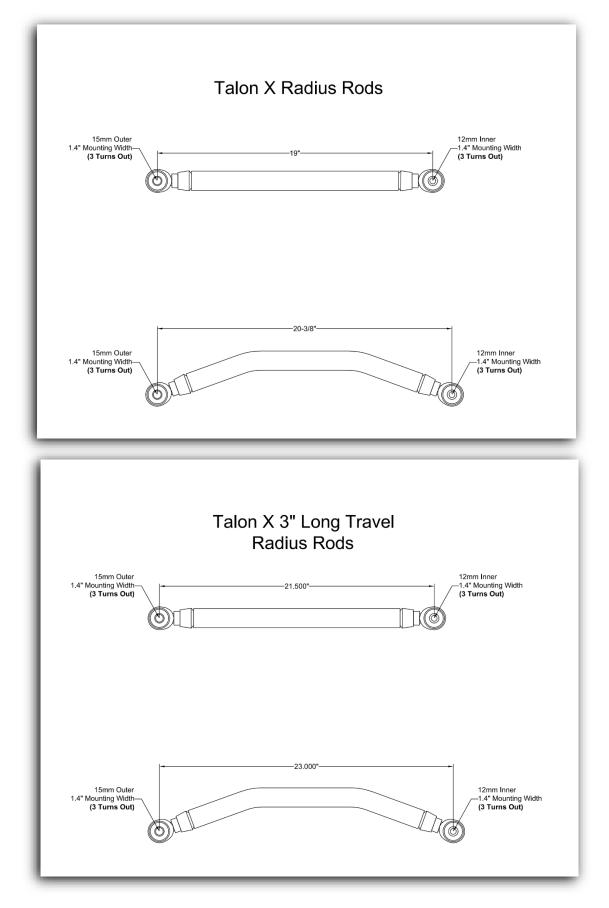
Once eye to eye dimensions are confirmed, install TTC Radius Rods onto the machine, using all factory mounting hardware.
