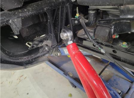
Using the stock hardware, install your new TTC Arms onto the machine and rear hub assembly.
