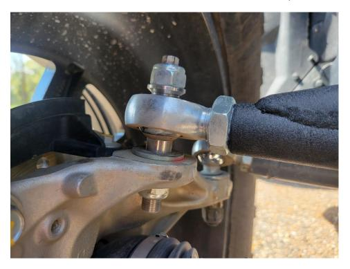
If you are running our heim style ball joint setup, first use a 10mm wrench to hold the pin, and tighten down the top locking nut on to the heim (no need to over tighten). Then insert the pin into the hub assembly and tighten the lower nut while holding the top of the pin with a 10mm wrench (no need to over tighten).
