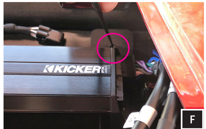
F. Using a scribe or punch, mark the location of the needed pilot hole on the passenger side of the tray.
