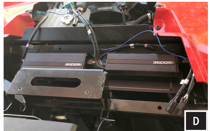
D. Place the amp tray into the mounting location by lining up the amp plate screw holes to the factory holes on the chassis.
