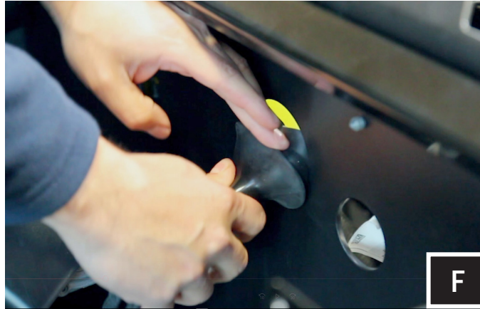
F. Unwrap the tape and pull the rubber wire grommet out of the firewall.
