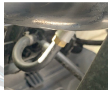
Image showing the boost controller vent line now routed into the AA intake tube via the brass barb. This is a fix for the line clogging.
