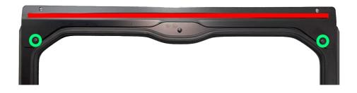
**Step 1:** Bolt the Windshield attachment to the front of the windshield using the two  $\frac{1}{4}$ -20 x  $\frac{5}{8}$ " bolts with washers on both sides, The location for the bolts is indicated by a green circle in the picture.
