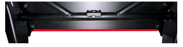
Step 5. Place 4 billet clamps onto the front vertical bars of roll cage (2 on each side). Position so that hump with the threaded hole is facing forward, and the clamping holes are positioned toward the center of the machine as shown. Use a 2" bolt with lock washer on each clamp by inserting into the unthreaded hole first, then into the threaded hole. Don't
