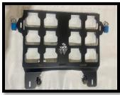
PARTS: (1) BENT MOUNTING PLATE
