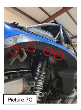
J. Remove your clamp. Align the fender extension with the contours of the OEM fender flare and clamp in place. (See Picture 8A thru 8C).
