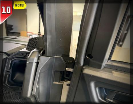
To access the hidden panel fastener, pull the side panel back just enough to reach and remove the push pin.
