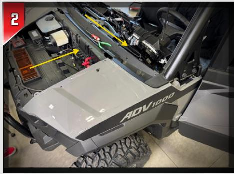
Locate the two (2) one (1)-pin harnesses: one labeled **Passenger | Pin-6** and the other labeled **Driver | Pin-7**. Starting from the hood side, feed the pins through the firewall and route them to the cluster connector.
