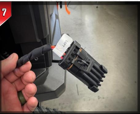
Grab the plug cap included with the taillight harness, then cap off the driver-side factory taillight harness.
