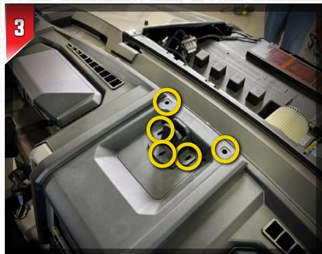
**Open** the windshield. Using a 10mm socket, **remove** the windshield latch on the dash by removing the three (3) bolts and two (2) push pins.
