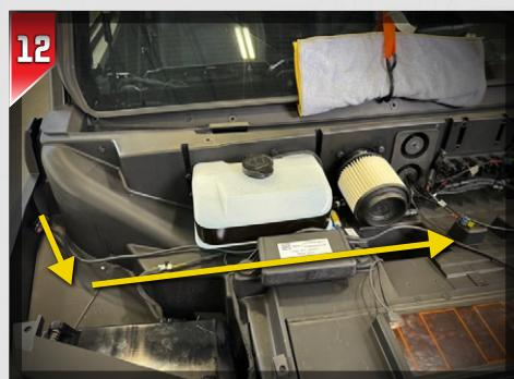
Grab the second **B-H3861** extension harness, plug it into the **B-H3112**, then finish routing it to the center of the hood compartment opening. The rest of the harness will hang out.
