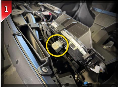
Unplug the instrument panel connector. Release the plastic clip located under the connector, then disconnect it. Be careful not to break the clip.
