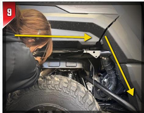
Now route the **B-H3112** harness toward the front of the vehicle, running it along the frame down into the rocker, securing it into place with zip ties.
