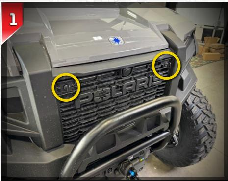
**Unlock** the two (2) twist-locking nuts on the front grille, then **lift** the grille up and out of the way.
