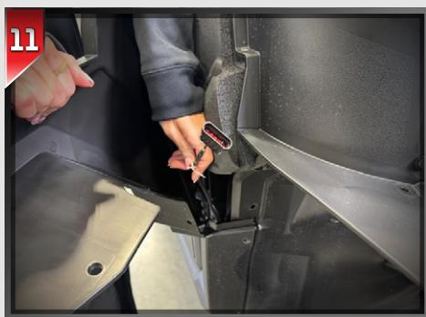
Now pull the **B-H3112** up through the front quarter panel. It may be easier to fish a guide wire down through the panel first, then use it to pull the **B-H3112** up.
