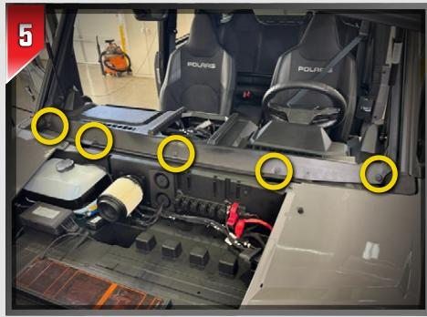
Remove the five (5) T-27 Torx screws from the top of the dash panel.
