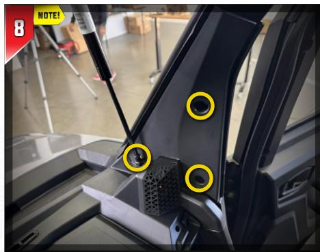
Remove the driver and passenger-side A-pillar covers. Release the windshield piston, then remove the two (2) T30 bolts and the 11mm windshield piston bolt.
