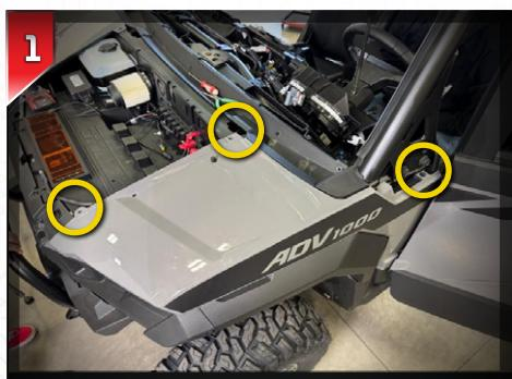
Remove the one (1) T40 bolt, one (1) T30 bolt, and four (4) push pins from both the driver and passenger-side fenders. Two (2) of the push pins are in the door jamb.
