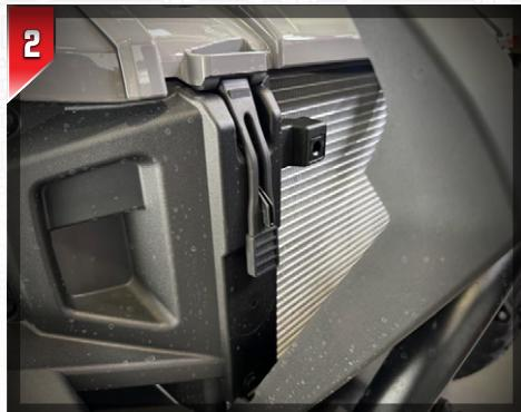
**Pull** down and out on the two (2) rubber locks that secure the hood, then **lift** the hood up and out of the way.
