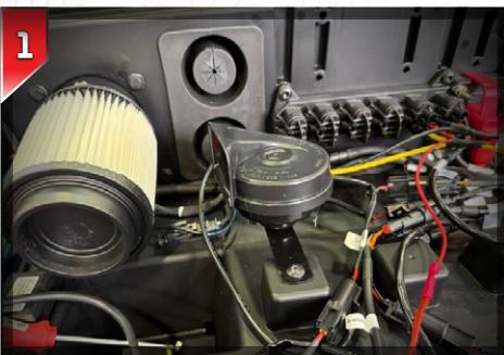
You can now mount the horn in a location that works best for your setup. In these instructions, the horn is mounted under the hood out of the way.
