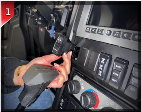
Choose the desired rocker switch location for your controller. Pop the cover out, then feed the **B-H2940** controller harness into the opening and snap the controller into place.
