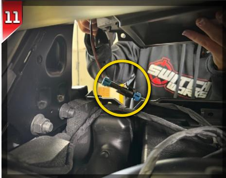
With all hardware removed, lift the end of the dash panel to disconnect the tweeters, if equipped.
