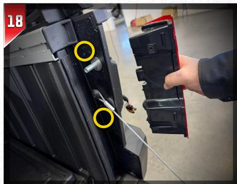
Move to the taillight and remove the two (2) T25 bolts securing the taillight. Pull the taillight out, then disconnect it from the factory harness. Repeat on the driver-side taillight.
