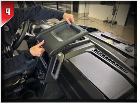
**Remove** the center top dash panel by lifting it up and out.
