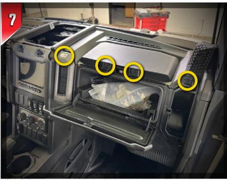
Remove the two (2) passenger-side HVAC vents. Open the glove compartment, then remove the two (2) plastic push pins next to the glove compartment latch. Also remove the plastic push pins behind the four (4) HVAC vents that were removed.
