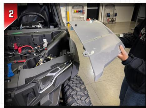
Carefully pry the fenders off. They are secured with plastic speed clips.
