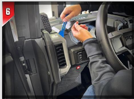
With a panel popper, remove the two (2) driver-side HVAC vents. They are secured with plastic speed clips.
