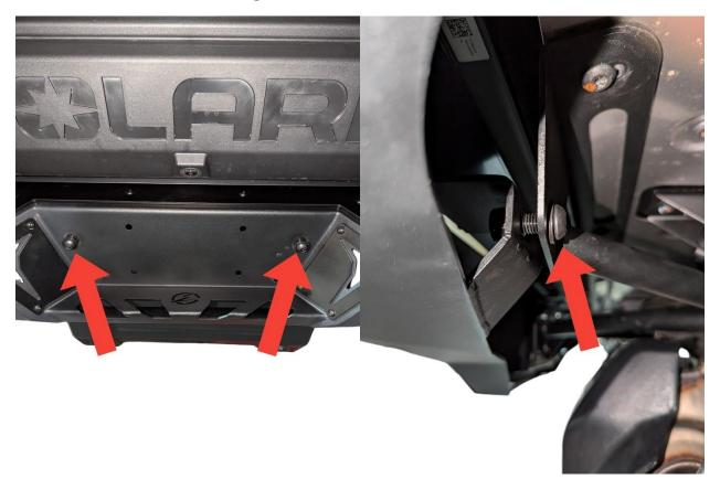
• Next set the outer bumper over the inner structure and then start the outer upper hex drive bolts in the license plate area with a 6mm hex tool and 17mm wrench to allow the bumper to sit on its own. From there install the lower inner and the 2x bolts that are on the outside in the wheel well area, once all the hardware is started you will need to align and level the bumper to the vehicles body and then tighten everything down starting with the inner bolts and working outward. Pay attention to
