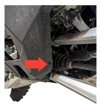
• Start off by removing the 4 torx bolts that secure the center portion of the bumper cover to the vehicle and then remove and set aside the enter section and the bolts removed, you will not need anything removed from this step. Remove the 4 torx bolts securing the outer portion of the bumper cover, these are located on the outside sections as shown in the picture above. Set aside the upper two bolts as they will get used later with the EOD bumper.
