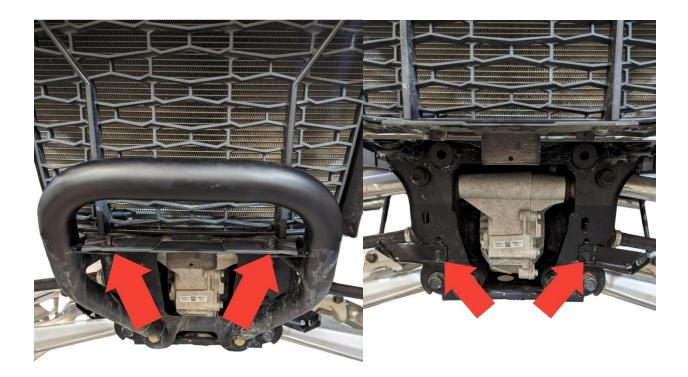
• Next remove the 2 plastic clips securing the lower portion of the grill to the bumper, these will not be needed anymore. From there remove the 4 factory 15mm bolts that secure the bumper to the vehicle, set aside the bolts for later use. Remove the 10mm bolts that secure the lower bumper cover brackets to the frame, these brackets and bolts are not needed anymore as well.
