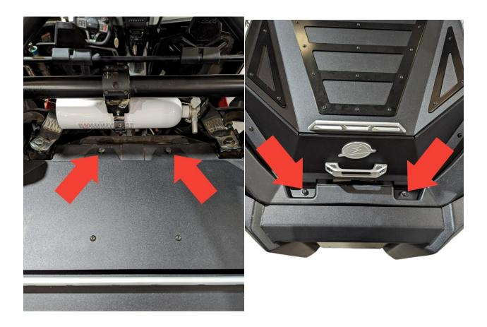
• Install two of the factory torx bolts loosely into the holes nearest to the seats and then install the 6mm bolts and washers into the two mounting holes towards the rear of the vehicle. Do not tighten down any of the hardware at this point.
