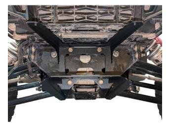
• Using the factory 15mm bolts removed earlier, mount the inner structure to the vehicle as shown in the picture above, torque down the bolts.
