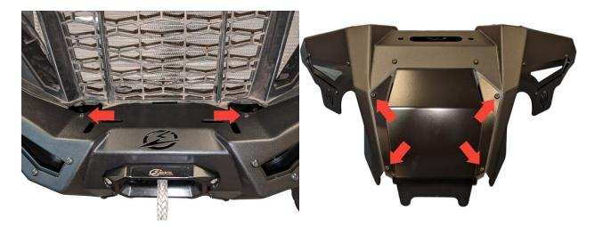
• Take the outer bumper and install it over the inner structure that is mounted to the vehicle making sure the fender and grill plastics go UNDER the outer bumper. Start the 2 top 5/32" hex bolts first then start the 4 hex bolts circled on the bottom section of the bumper, refer to the pictures above if needed. Once all 6 hex bolts are slightly threaded in, they can now be tightened down working from the center 2 bolts, upper 2 bolts and finally the lower 2 bolts.
