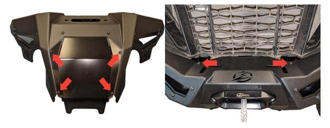
• Separate the EOD bumper's inner structure from the outer bumper by removing the hardware with arrows pointing to them in the pictures above with a 5/32" hex tool.
