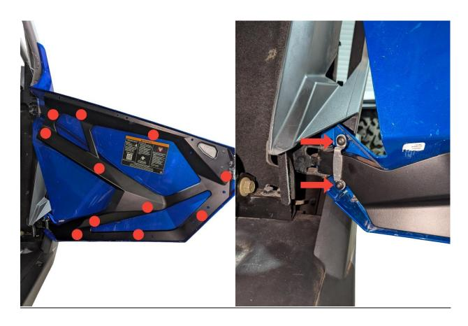
Start off by opening the door and removing the aluminum strap that wraps around the lower door hinge with a T25 torx, next remove the remaining 9 T40 torx bolts. When all the hardware is out shut the door and then lift the outer door skin off the door frame. No hardware taken off will be used furthermore.
