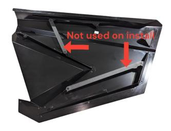
• Lay the EOD door skin on a clean scratch free surface and remove all the hardware and two braces per skin, keep all the hardware and go ahead and discard the braces that were just removed.
