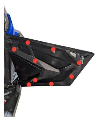
Carefully lower the door skin over the top of the door frame with the bottom section of the skin slightly angled out to assist in installation, once it is lowered down and on top let the bottom swing down and get a couple holes lined up with a couple bolts started. Go around the rest of the door skin and loosely install all the remaining removed bolts.
