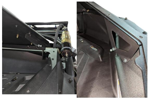
• Next bolt the ball studs for the lift struts to the interior of the box as shown with the upper ones facing to the outside and the lower ball ends facing to the center of the vehicle.
