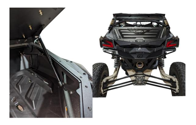
Once the ball ends are tightened down the lift struts will be installed with the body of the struts up and the rods coming out of the bottom, see attached picture if needed. Perform a final check over of all the work completed and enjoy another great product from Elektric Offroad Designs!
