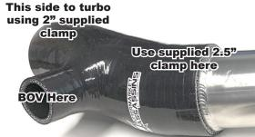
Use straight coupler and supplied 2.25" clamp here along with the factory 2.25" clamp
