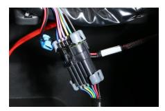
**11.** Install Power Harness. Unplug the AUX power connector under the dash, plug our adapter into it and then plug back into the power outlet. It goes inline. Plug the other two pin connector into the ATS-CM control unit.
