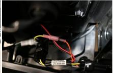
6. Run the green wire to the passenger side taillight, follow the factory harness, secure harness with provided cable ties. Plug the green wires into the previously installed adapters orange wire.
