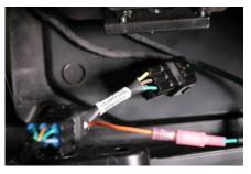
7. Install the front adapters to use the factory amber turn lights. Unplug each headlight and plug the adapters in-line.
