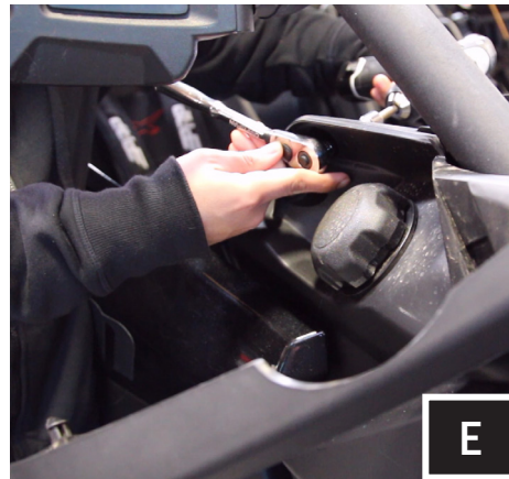
E. Remove gas cover on the passenger side to expose a 10mm nut. Unscrew with a wrench and T30 torx driver.
