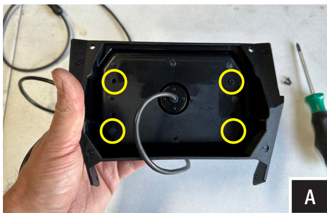
A. Insert the LCD Touch Button Controller cable thru the RZ5 controller dash panel center hole and use the 4-40 fine thread cutting screws (x4) to secure it on the dash panel.
