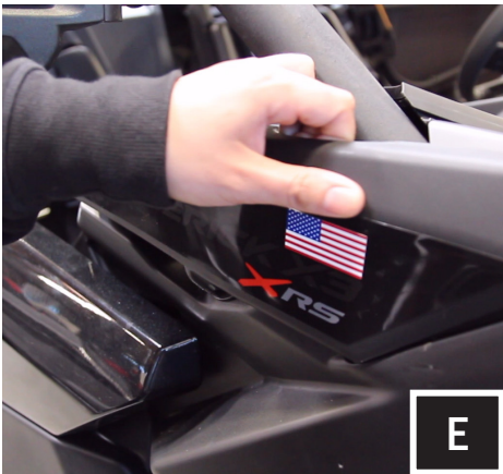
E. Remove gas cover on the passenger side to expose a 10mm nut. Unscrew with a wrench and T30 torx driver.
