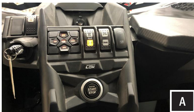
A. Reach behind the center panel and remove the factory Start/Stop button by unscrewing the retention nut behind it.
