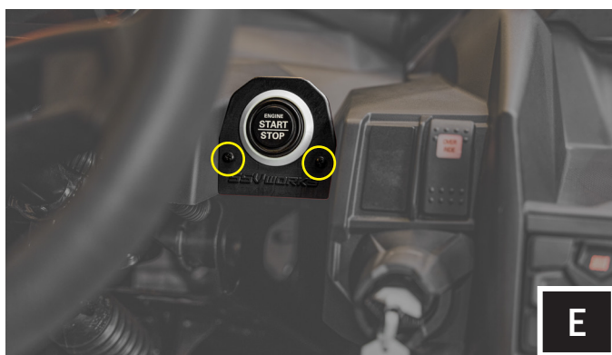
E. Mount the assembled Start/Stop relocation assembly using the two M3 screws (B-S1357).
