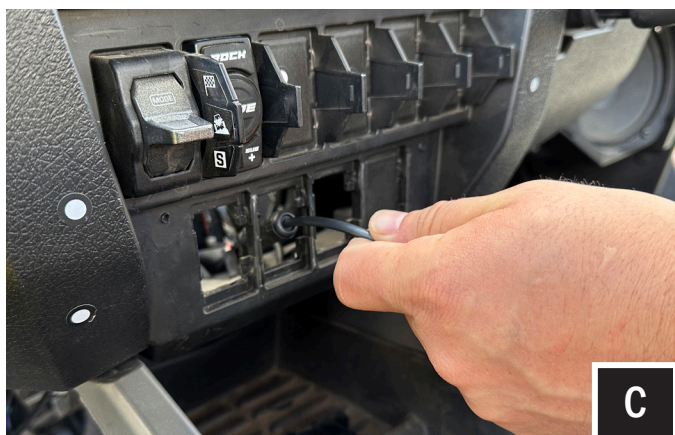
C. Fish thru the LCD Touch Button Controller cable into the dash cavity.
