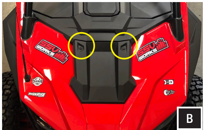
B. Remove the (2) T40 torx screws and set the hood panel aside.
