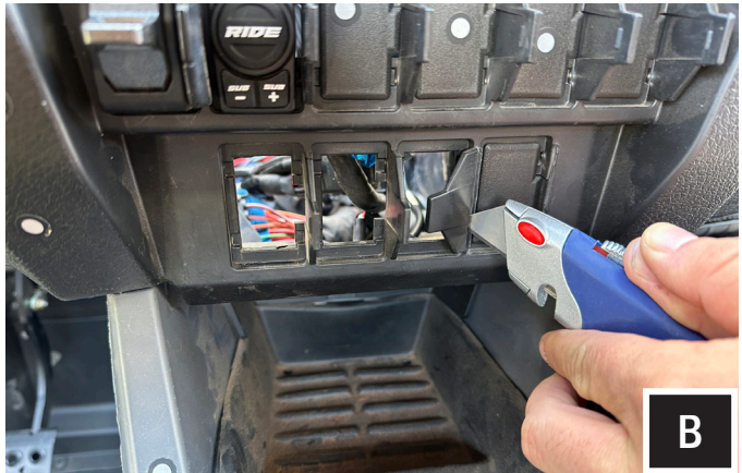
B. Carefully cut off the bottom row rocker panel separator fins of the center dash.
