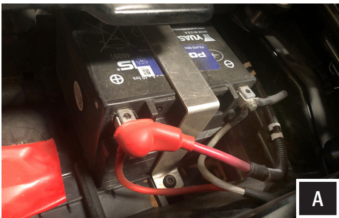
A. Using a 8mm wrench. Disconnect the negative battery cable from the battery.
