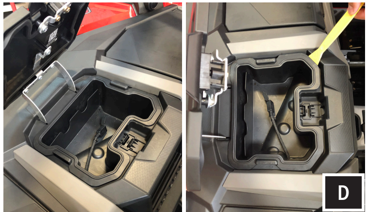
D. Open the top-center dash compartment and lift to remove the compartment tray. We recommend using a panel tool to assist releasing the tray from the compartment. Once the tray is separated from the compartment, pull out the USB cable from the tray, set tray to the side.
