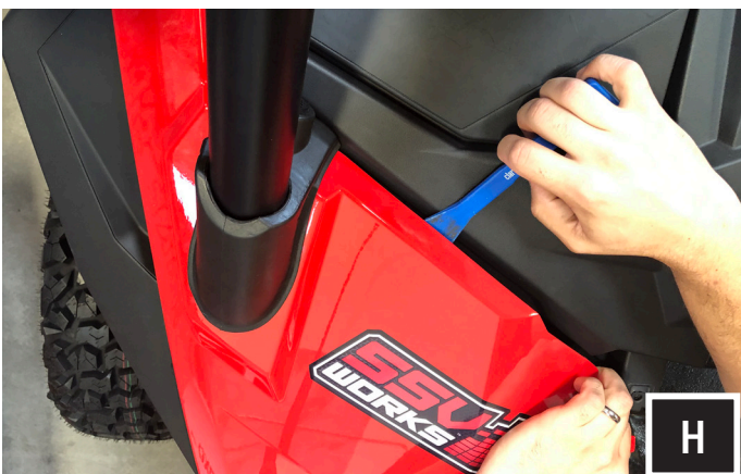
H. Use a panel to aid in lifting the fenders to release the top dash panel.
