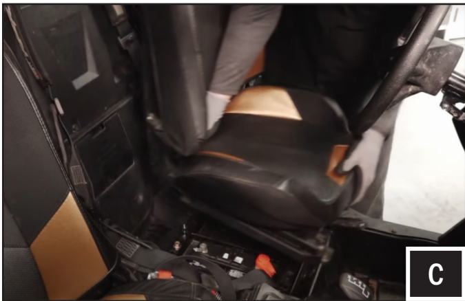
C. Run the power and ground wires from the ALPHA12 kit to the battery location. The battery is located under the driver seat on 2 door models and under the rear driver seat in 4 door models.
