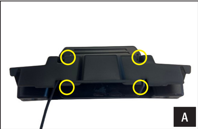
A. Insert the LCD Touch Button Controller cable thru the KRX upper dash controller mount center hole and use the 4-40 fine thread cutting screws (x4) to secure it on the dash panel.
