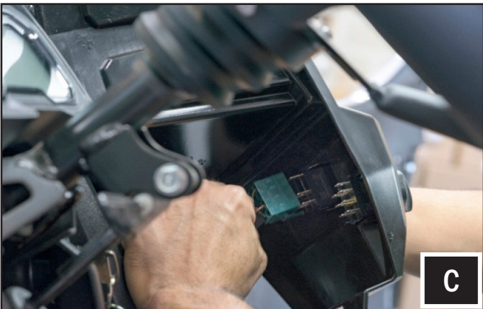
C. Lift the dash panel and unplug the drive selector and gear selector switch connectors.
