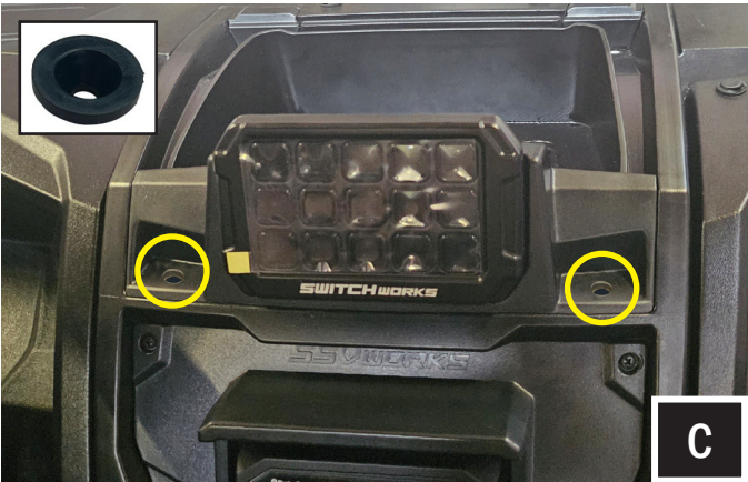
C. Line up the dash panel in place and drill holes on the front dash using the drill guide as a template.
