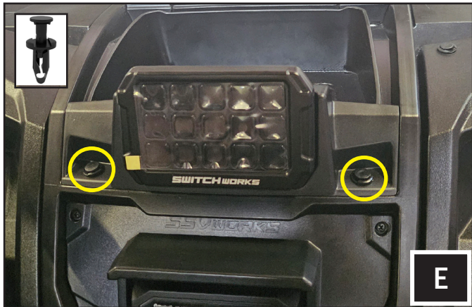
E. Use the provided push-in style snap rivets to secure the upper dash controller mount panel to the dashboard.
