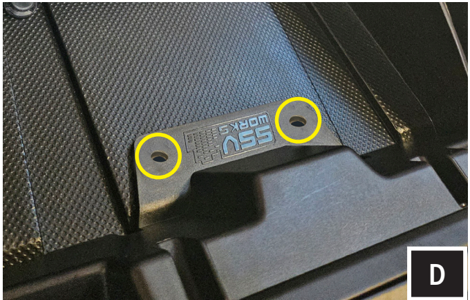
D. Drill holes on the top dash using the drill guide as a template.
