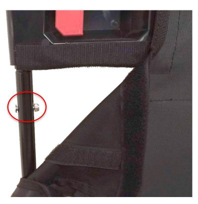
**8.** Attach Upper and Lower door frames using M6x25mm button head fasteners and corresponding M6 locknuts. The locknut should be on the inside of the door frame as shown.
