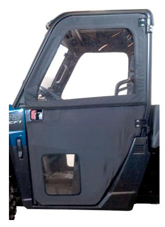
**20.** Move the door into the "closed" position. With the window down, you can make adjustments to the striker bolt and plate to ensure the door fits properly.
