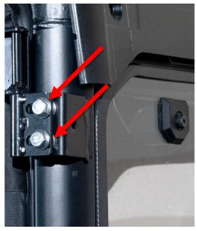
**1.** Install Upper Hinge Plate and Upper Backing Plate onto the mounting location at the upper rearward part of the ROPS structure. Install using M8x20mm fasteners and M8 Washers as shown. Do not fully tighten at this point as adjustments will need to be made when hanging the door structure.
