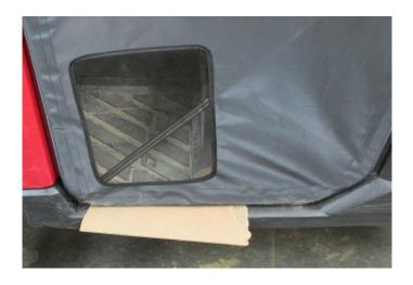
**21.** We have found that placing a piece of scrap cardboard at the bottom edge as shown will help line up the door so that it will not drag on the bodywork when the door is finished being adjusted.
