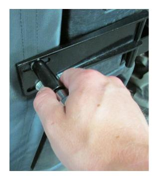
**24.** Move the door back into the closed position, again pressed firmly against the gasket on the bodywork. This may require you to move the striker assembly up or down in order for the latch to fully engage. At this point tighten the door plate bolts just enough to keep the door from sliding forward and back.
