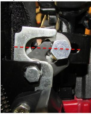
**25.** Shown above is the correct alignment for the striker bolt and latch just before the door is closed. The bolt should line up in the center of the relief in the latch. This will allow the door to close smoothly.
