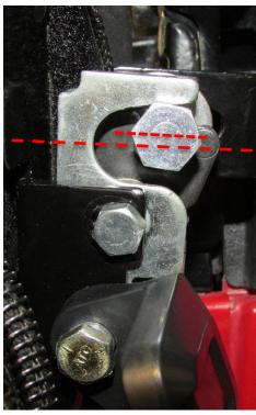
**27.** In the image above the striker is aligned incorrectly. Note the latch is not fully closed and the striker bolt is not aligned in the center.
