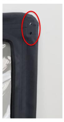
**16.** Holes need to be cut in door textile panels in order to mount the Upper and Lower Sliding Hinges. **Ensure textiles are tight and fit as desired before marking and cutting holes.** Take a sharp scribing tool and punch a small hole through the textile indicating the center of the slot. Take a razor blade and carefully cut out the small amount of textile so that the supplied M8 bolt may pass through the plate and the textile. Repeat this process for the lower mounting location.
