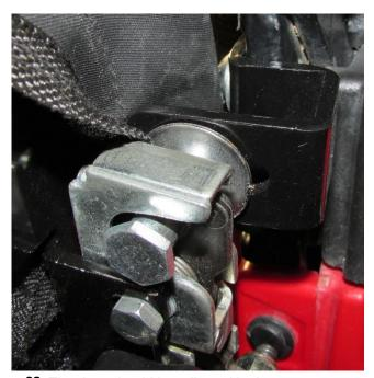
**28.** The door should be adjusted in the forward/rearward direction so that the striker bolt head does not contact the latch. The image above shows the correct positioning of the striker bolt.
