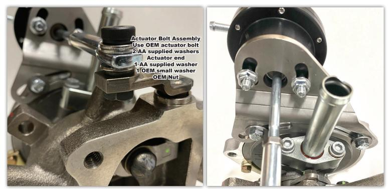
Standard actuator kits come with a stiffer 7-11psi spring option. Swapping the spring is easy. If needing to use the stiffer spring to achieve proper crack pressure, simply remove the 6 bolts holding the billet actuator together; keeping in mind there is some light spring pressure. Remove the assembly inside and swap the spring. When bolting back together, make sure you center the inner seal as best as possible.
